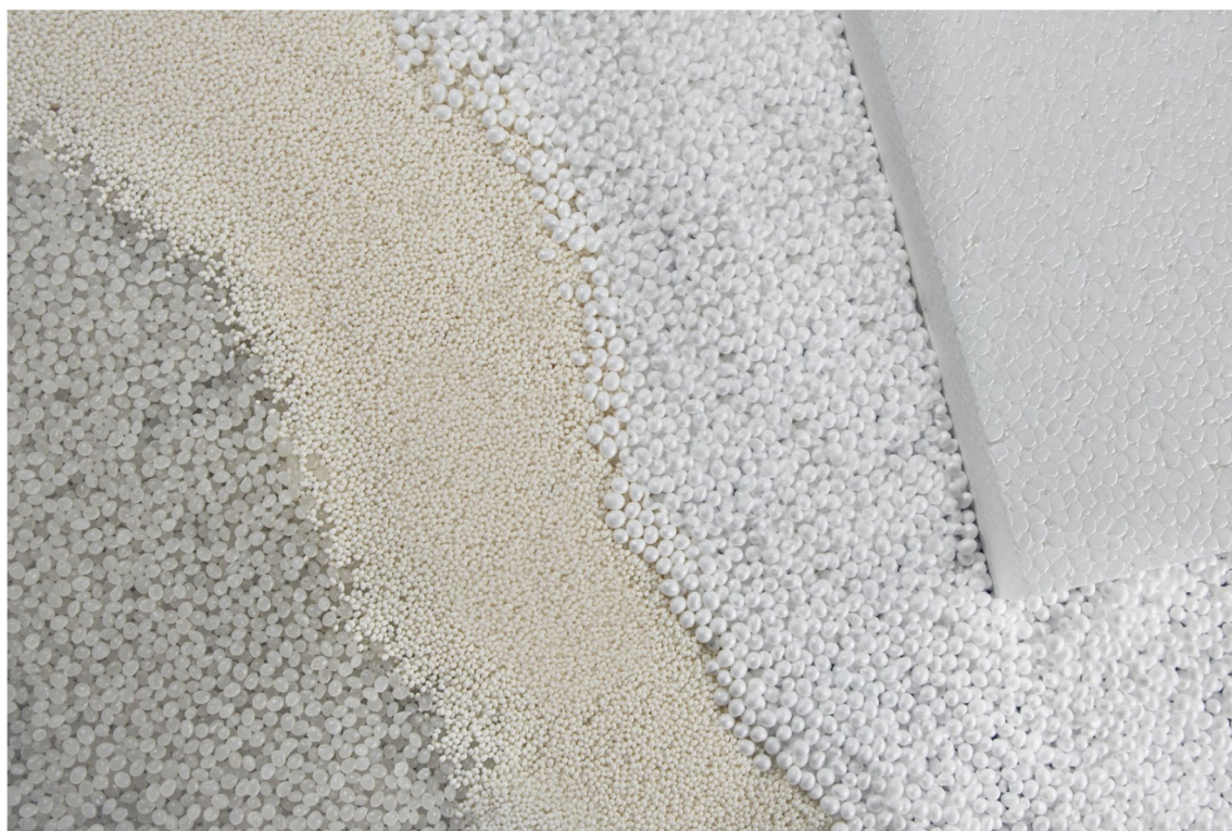
FIGURE 1 From left to right: PLA granule, PLA blowing agent containing granule, pre-expanded PLA beads and sintered PLA bead foam plate [Color figure can be viewed at wileyonlinelibrary.com ]
