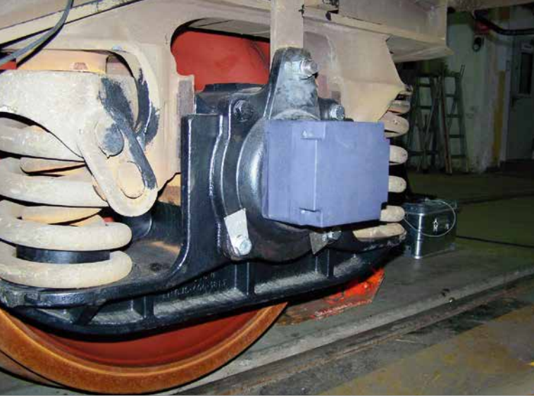
Nachhaltige Energieversorgung von intelligenten Sensoren an Güterwagen dank Schwingungsenergiewandler. Sustainable energy supply of intelligent sensors on freight cars thanks to vibrational energy converters.
